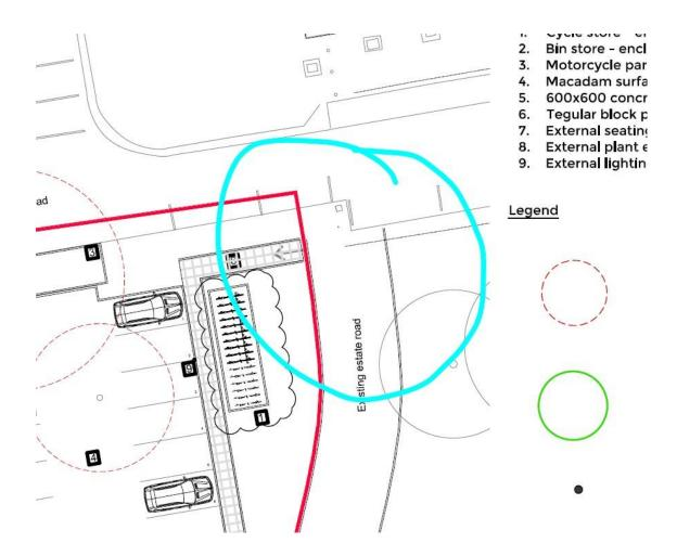
The layout of the existing estate road does not appear to accurately represent what is on site – particularly the bell mouth on the east side of the access:
